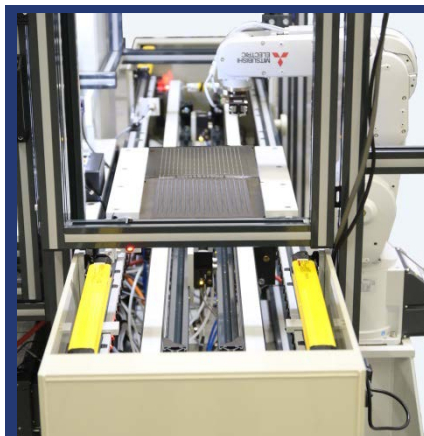
6-station linear transport unit for holding pallets
