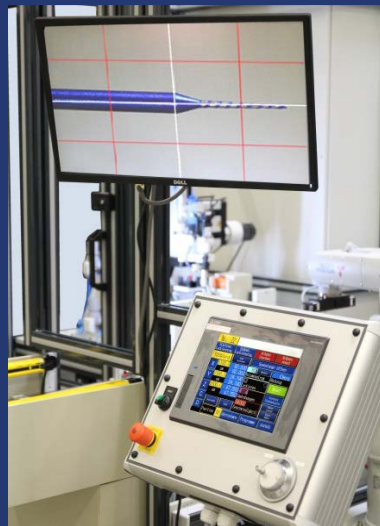
Monitor and Touch screen-operators terminal for process surveillance and control
