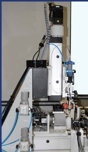
Varnishing unit with four-axes guidance and volumetric dosing system VDS-145
